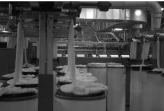
Cotton rovings being drawn up to be made into cotton thread for weaving.
